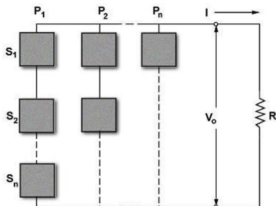
Fig. 2. A typical TEG configuration with series/parallel connected modules.
