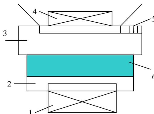
Fig. 3 TEG components: 1, 4 - fans, 2 - cold radiator, 3 - hot radiator, 5 output lead for the generated electric power, 6 - insulation
