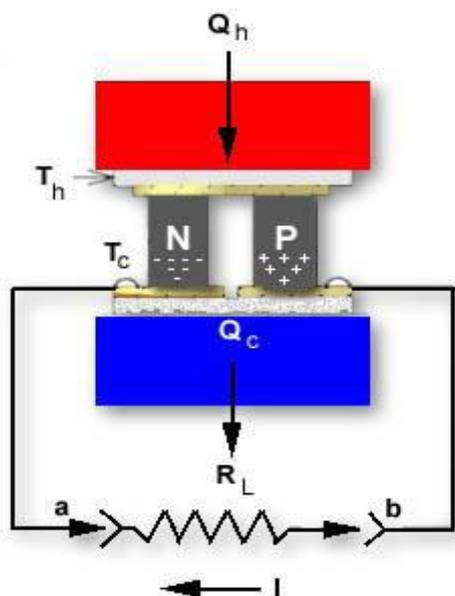
Fig. 1 A single thermocouple;  $T_h > T_c$
