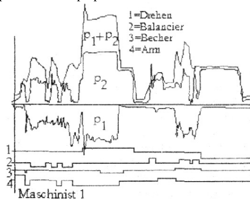
Fig. 1. Instantaneous power on the working cycle for an excavator of 1.2 m 3 bucket capacity
