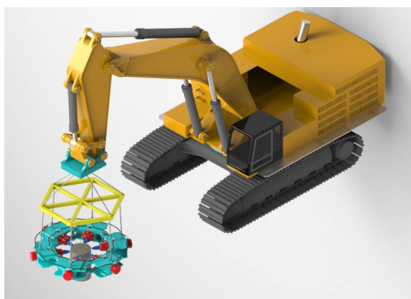
Fig.6 The -3D model of- thepile breaker attached to the -excavator arm
