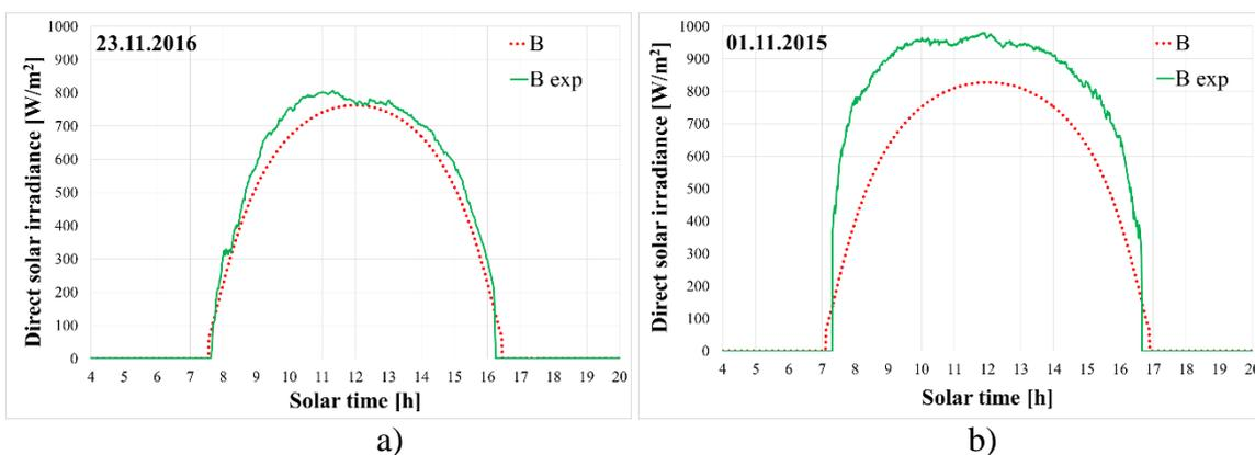
Fig. 4 Simulated and experimental direct solar irradiance in the two selected clear sky days
