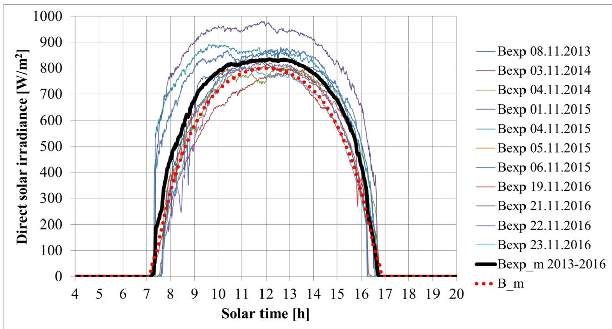
Fig.3 Simulated and experimental direct solar irradiance: November 2013-2016
