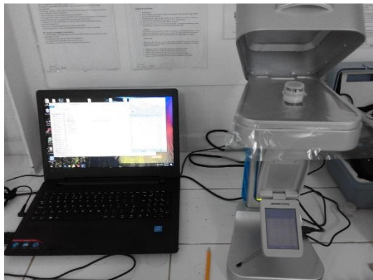
Fig. 1. Portable Genius XRF spectrometer used for the investigation of industrial sludge samples
