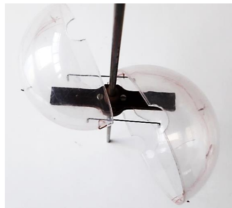
Fig. 5. Experimental Model for VAWT with hemispheric cups
