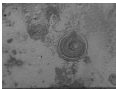
Fig. 7. Localized corrosion caused by a pore, 1:1
