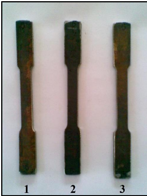
Fig. 2. Macroscopic images of the 1010 samples used in the mechanical tests: 1) non-service specimen, 2) service horizontal boiler specimen and 3) service vertical boiler specimen
