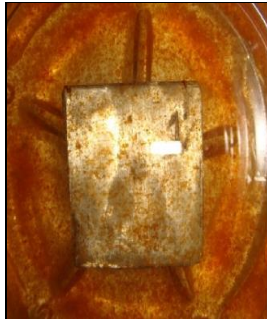
Fig. 5. Macroscopic image of the tested specimen in the corrosive environment during the weight loss analysis
