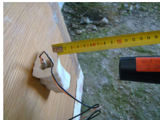
The distance between the electrically detonating cap inserted in an amount of 100 g plastic explosive and disrupter is about 10 cm
