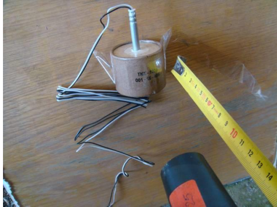
The electrically detonating cap assembly is inserted into a 100 g of TNT body at a distance of 10 cm from the disruptor
