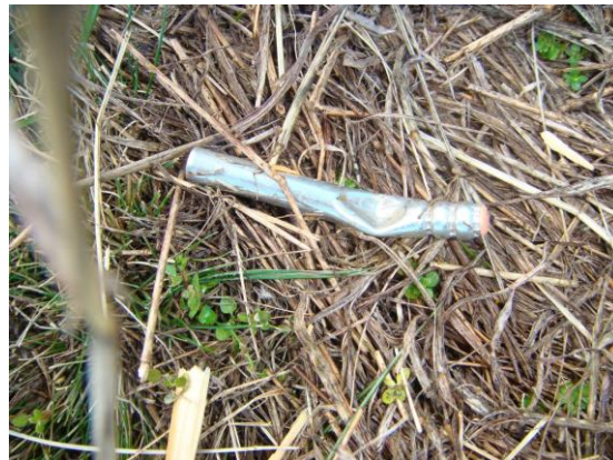
Electrically detonating cap deformed after disruption
