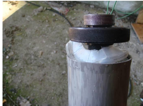
Compensating cover deformed after disruption
