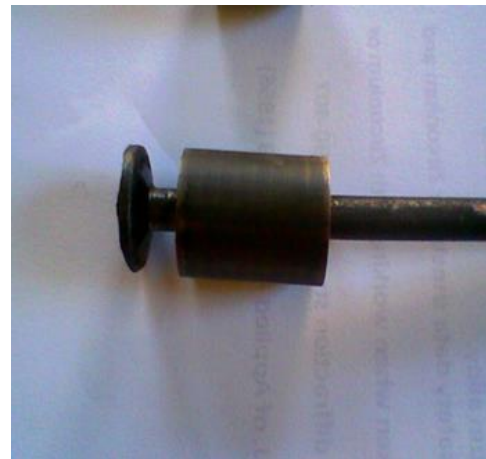
Fig. 5. Aspects of the stages of hot extrusion molding to a diameter of 10 mm of the blank having 18 mm diameter and 35 mm length; the new blank of \Phi 10 \times 35 mm was subject to heating at 850 °C then hot extruded at the \Phi 5 mm diameter. Finally, the \Phi 5 mm extruded blank was cold rolled to a diameter of \Phi 3 mm
