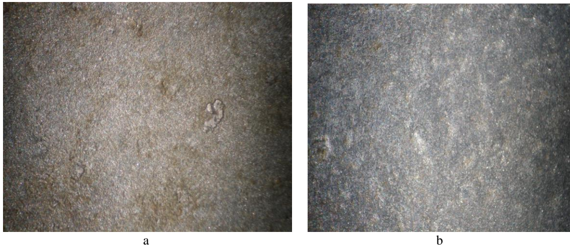
Fig. 13. Surface appearance of covered NbC samples after corrosion a) 6 μm; b) 8 μm
