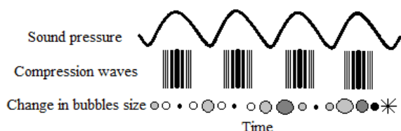
Fig. 1. Compression and expansion cycle of ultrasound [4]
