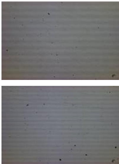
Fig. 1. Microscopic appearance (optical microscopy without metallographic attack, magnification X50) of the Co-Cr alloy samples (ADORON LX40626) delivery/marketing state of alloy [5]
