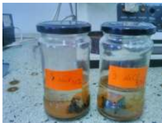
Fig. 1. Samples tested for corrosion in NaCl 3.5% saline solution
