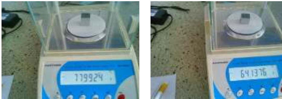
Fig. 2. Weighing samples subjected to the corrosion test
