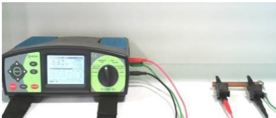
Fig. 5. Electric insulation resistance measurements
