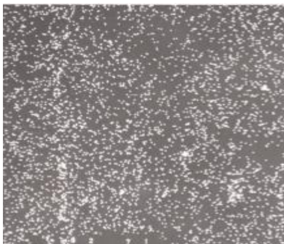
Fig. 9. Si Distribution, X300
