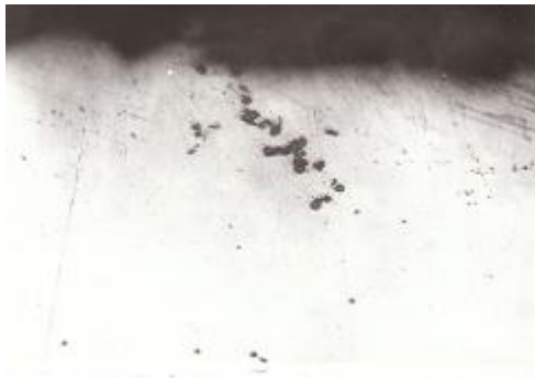
Fig. 2. Non-metallic inclusions on the oscillation mark – charge 936884 – X250
