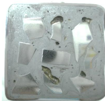
Fig. 4. Sample Ti6Al4V attacked with cu Kroll reagent
