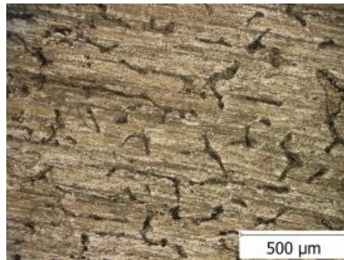
Fig. 6. Spots of burned emulsion with atypical forms
