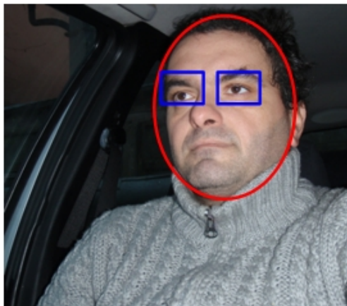
Fig. 4. Face detection and eye opened detection
