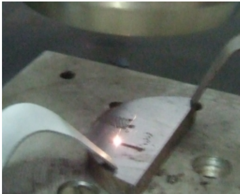
Fig. 4. Interaction of laser radiation with sample and intense sparks due to interaction
