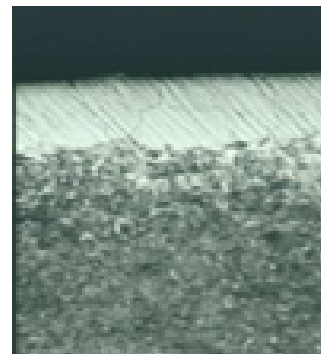
Fig. 8. Superficial layer thickness before wear tests, for of T13' treatment regime (x100) (with a.c. magnetic field regime)
