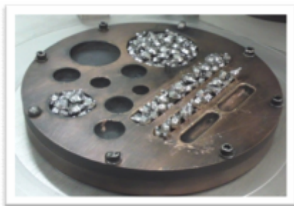
Fig. 3. Commercial Co-Cr-Mo alloy prepared during elaboration process
