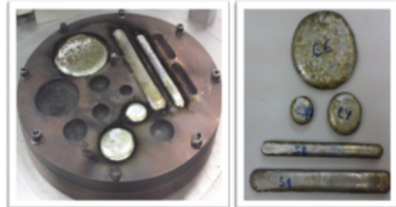
Fig. 5. Commercial Co-Cr-Mo alloy after solidification – casting samples
