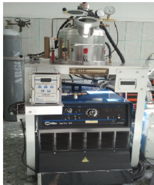
Fig. 2. Remelting installation with electric arc, under vacuum, type MRF ABJ 900
