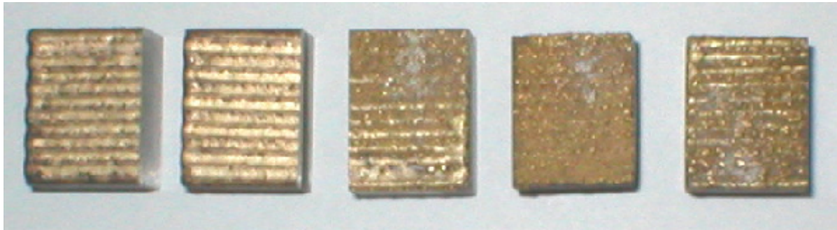
Fig. 2. Surface of samples cladded by thick layers of aluminum bronze
