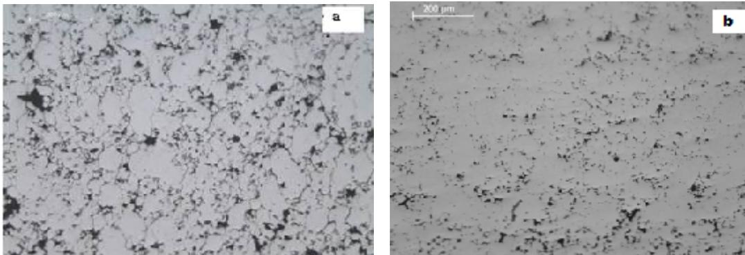
*Fig. 1. Image of the microstructure of carburized samples, unetched, 200x: a) P<sub>1</sub>, b) P<sub>2</sub>*
