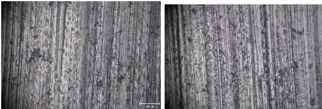
**Fig. 3.** Optical photomicrographs of worn surfaces for carburized in fluidized bed samples (x200): a) P<sub>1</sub>, b) P<sub>2</sub>
