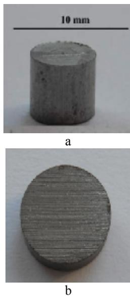
**Fig. 4.** Aspect of initial and worn surface after the abrasion test of carburized in fluidized bed specimens
