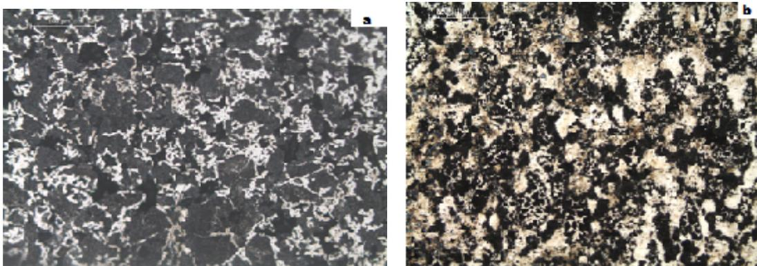
*Fig. 2. Image of the microstructure of carburized samples, etched Nital 2%, 200x: a) P<sub>1</sub>, b) P<sub>2</sub>*
