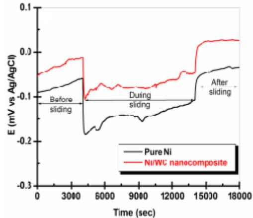
**Fig. 8.** Evolution of the open circuit potential recorded before, during and after sliding tests of Ni/nano-WC composite and pure Ni coatings in the boric acid and lithium hydroxide solution at 1 Hz, 200 µm, 10000 cycles for the normal force of: 5 N [L. Benea and group - unpublished work]
