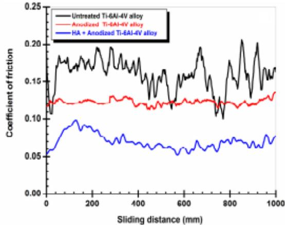
**Fig. 9.** Evolution of the friction coefficients versus sliding distance for (—) Untreated Ti-6Al-4V alloy surface; (—) Anodic nanoporous TiO<sub>2</sub> film surface and (—) hydroxyapatite electrodeposited into nanoporous TiO<sub>2</sub> layer, at normal forces of 800 mN, sliding frequency - 1 Hz and sliding cycles - 1000
