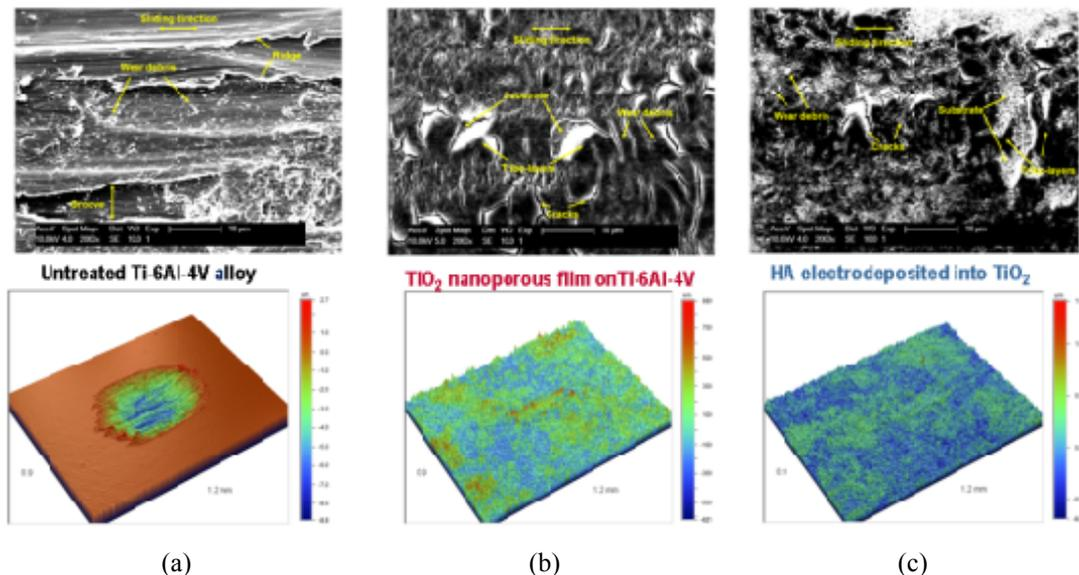
**Fig. 10.** SEM images of the wear tracks in the central region and 3D views obtained by non-contact profilometry of the wear tracks after reciprocating sliding tests ( $F_N=800$  mN, displacement amplitude 500  $\mu$ m, 1 Hz and 1800 sliding cycles) performed in artificial saliva for: (a) untreated Ti-6Al-4V alloy surface; (b) Anodic nanoporous TiO<sub>2</sub> film surface and (c) hydroxyapatite electrodeposited into nanoporous TiO<sub>2</sub> layer surface
