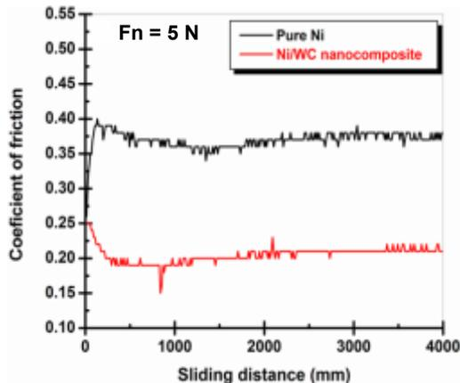
**Fig. 7.** Evolution of the friction coefficient of Ni/nano-WC composite and pure Ni coatings during fretting wear tests performed in wet conditions (solution with LiOH and H<sub>3</sub>BO<sub>3</sub>) at 1 Hz, 200 µm, 10000 cycles for the normal force of 5 N [L. Benea and group - unpublished work]
