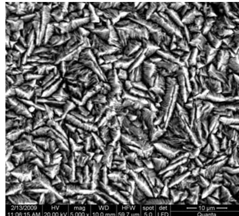
Fig. 6. SEM surface morphology of epoxy resin/Zn composite layers obtained at 3A/dm 2 with mean diameter particles size in electrolyte solution 6 – 10 \mu m (x 5000)
