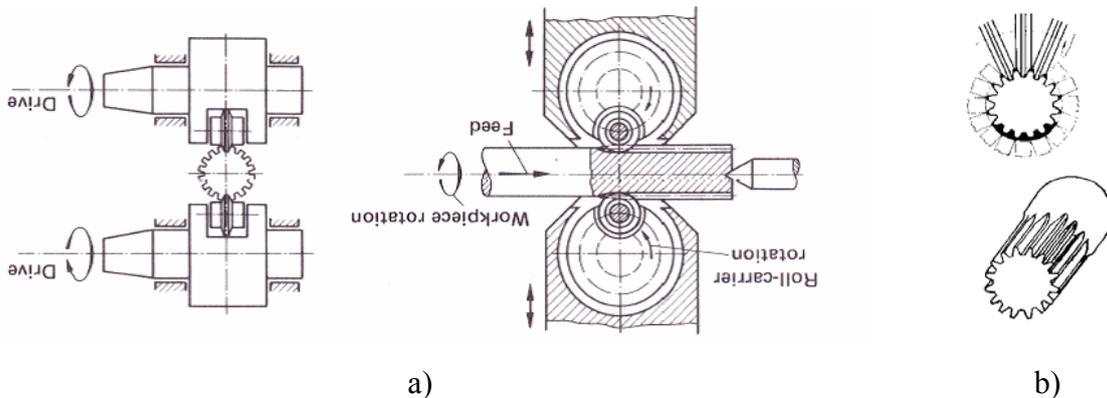
**Fig. 3.** Longitudinal rolling of grooved parts with: a) superficial pressing [4]
