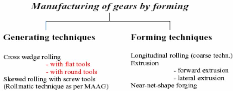
**Fig. 2.** Various processes for gear manufacturing [1]
