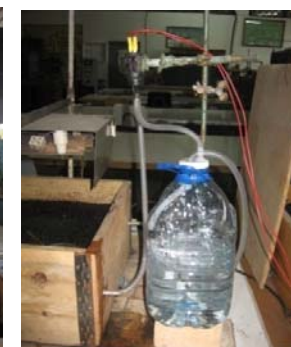
Photo 6 Water buffer tank
