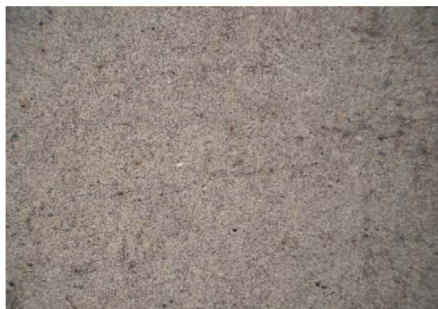
Fig. 15. Microstructure obtained after the quenching + high annealing treatment (improvement) for the steel 42MoCr11 - sorbite (X100)
