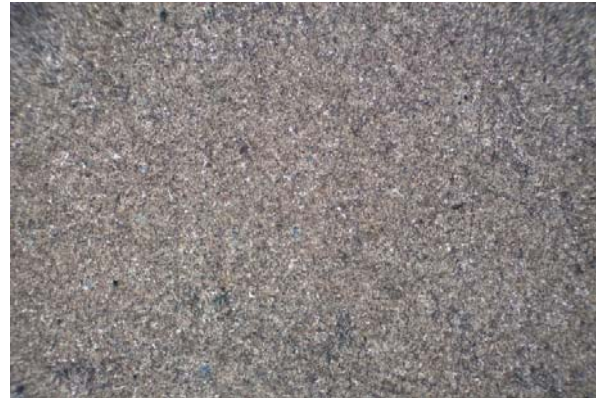
Fig. 7. Microstructure obtained after the normalisation treatment for the steel 42MoCr11-ferite+perlite (X100)
