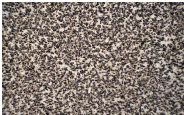
Fig. 10. Microstructure obtained after the quenching treatment for the steel 40VMoCr11– martensite + rezidual austenite + troostite (x100)
