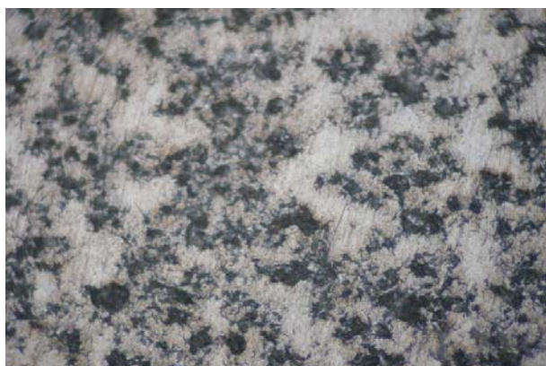
Fig. 12. Microstructure obtained after the quenching treatment for the steel 40VMoCr11 – martensite + rezidual austenite + troostite (X500)
