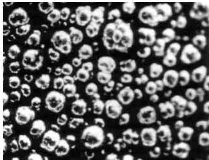
Fig. 1. Cobalt layer; current density: 570A/m 2 ; 50X
