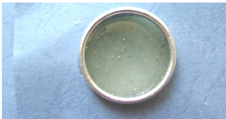
Fig. 3. Glass with nickel oxide after thermal treatment
