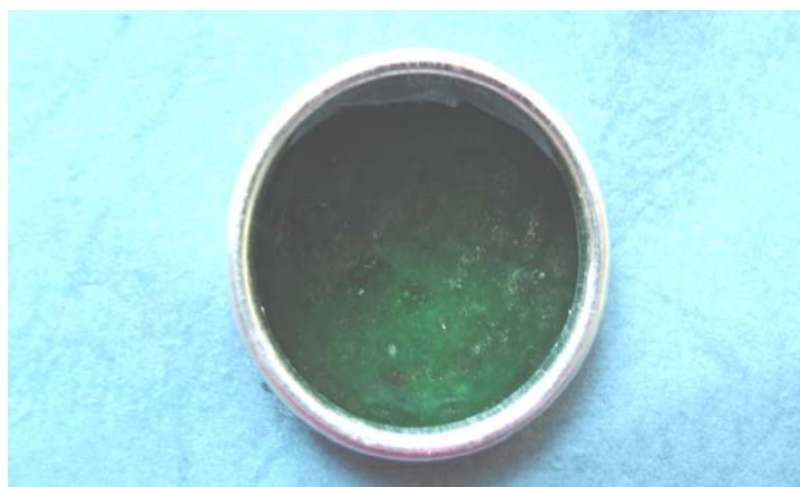
Fig 2. Green glass obtained by adding in charge of iron oxide
