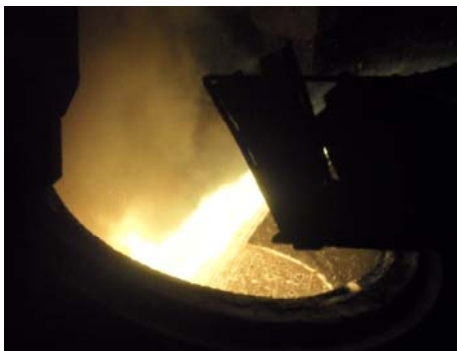
Fig. 5. EAF tapping in ladle
