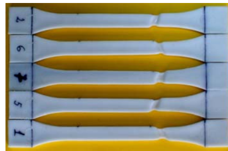
a) set of five samples, after being tested
