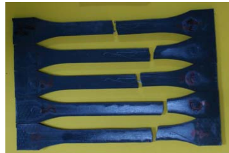
Fig. 7. Stress-strain curve (left) for PBT and tested samples (right)
