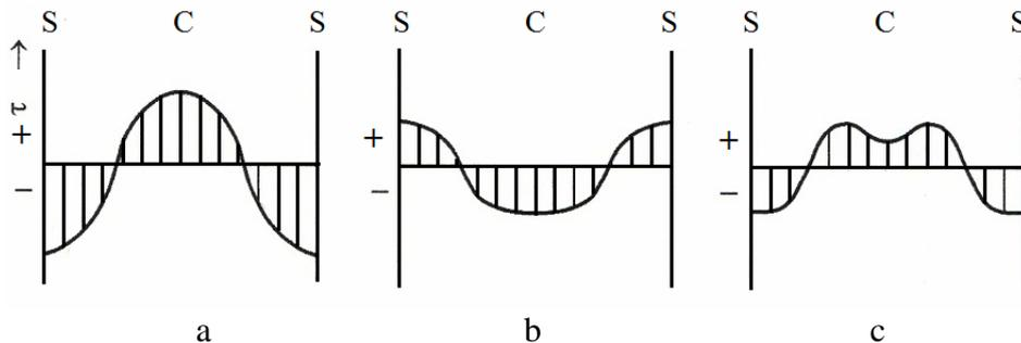
**Fig. 1.** Distribution of the stresses in the superficial layer: a-thermal stress; b-structural stress; c-resultant stress.
