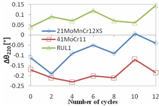
Fig. 6. Distribution of  $2(\Delta\theta)_{220}$  vs. testing cycles
