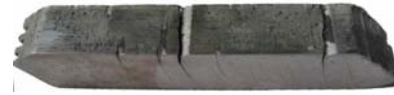
Fig.8. Cracking during ECAP process. Cracks start from upper surface of the billet.
