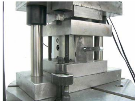
Fig.2. Experimental device for ECAP.
