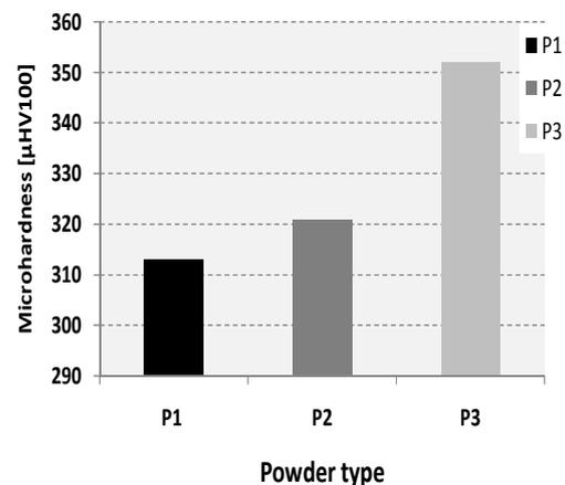
**Fig.6.** Vickers microhardness values of the carburized samples.
