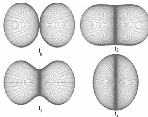
**Fig.1.** The schematic of two powder particles during sintering, carried out using finite element method at different sintering times,  $t_0 < t_1 < t_2 < t_3$  [7].
