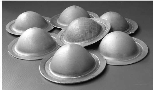
Fig. 6. Hemispheres obtained through free-bulging under low pressure.
