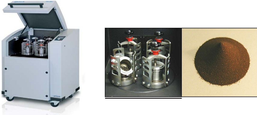
Fig. 3. Retschmaschine and steel vials for preparing mixed powder of Cu7Ag 0.05Nb for compressed rods.
