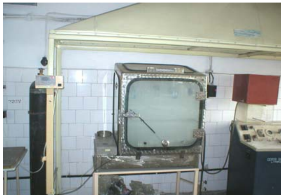
Fig. 3. Salt spray chamber used for testing corrosion resistance.
