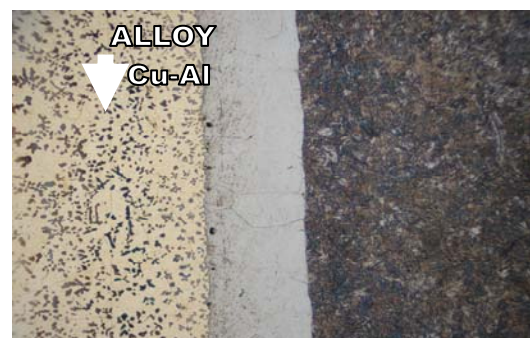
Fig. 9. Microstructure of bimetal after exposure to metallographic attack (X200)
