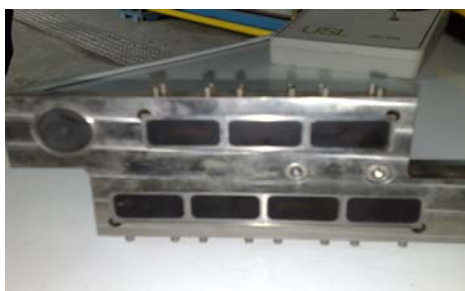
Fig.2. Head transducers, seven unfocused transducers (rectangular) and a focused transducer (circular shape)
