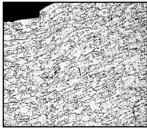
Fig. 7. Microstructure in the cutting zone at the beginning of the cutting process (Nital 2%, \times 200 )
