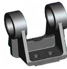
Fig. 10. Support made of cast semi-product.
