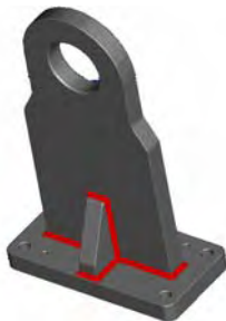
Fig. 8. Support made of welded semi-products.
