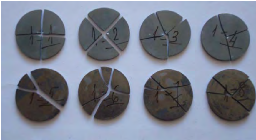
Fig.5. Specimens from reinforced titanium ceramic – type 1 after fracture.
