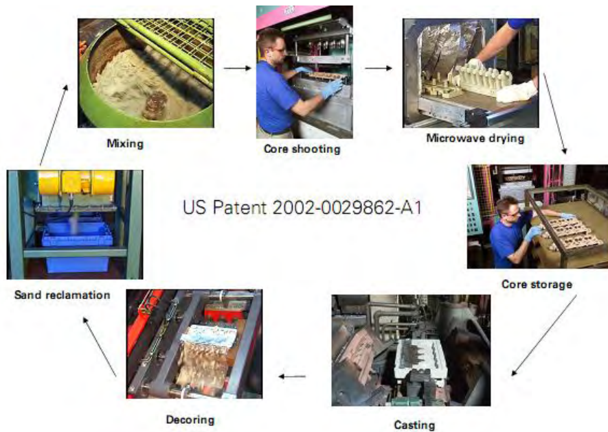
Fig. 1. Castings production using the AWB process.
