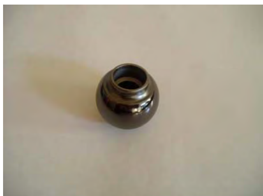
Fig. 5. A selection of glass-carbon coated ceramics produced with the setup described.
