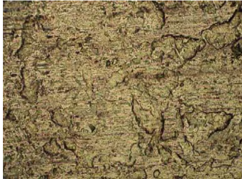
Fig. 1. The surface aspect of the blank assay x200 (before the corrosion)
