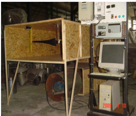
Fig. 6. Experimental wind tunnel and system for variable wind speed
