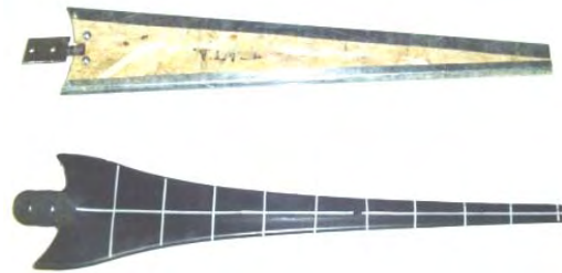
Fig. 7. Experimental variable surface blade and original AirX blade
