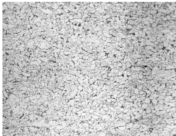
Fig. 1. Microstructure of normalized RV52 steel plates Magnified x 100
