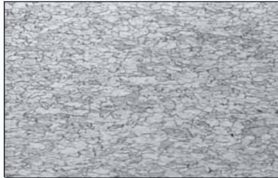
Fig. 8. The steel macrostructure after 140 days of natural ageing in longitudinal section (magnification 100x).
